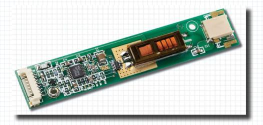
The new "A Series" modules are designed as a higher performance near drop-in replacement for those customers and applications currently using the LXMG1617 and LXMG1618 inverters.
