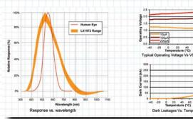
Internal temperature compensation allows dark current to be kept below 200nA over the full specification temperature range (-40 to +85°C), providing high accuracy at low light levels. Usable ambient light conditions range is from 1 to more than 5000 Lux.
