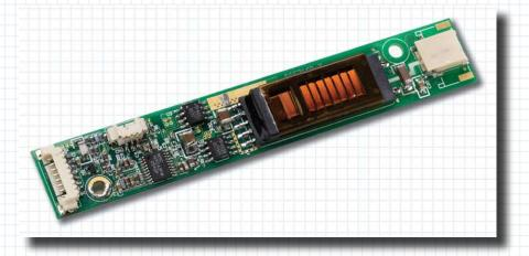
The LXMG181X Series, available in 5V and 12 V Input, is an enhanced offering to run single CCFL lamp displays. It integrates the latest, most intelligent and efficient Microsemi CCFL ICs.
