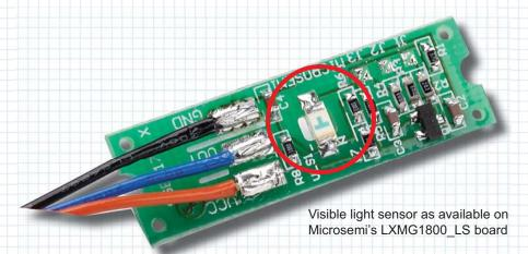
The LX1972 and the LX1972A are low cost silicon light sensors with spectral response that closely emulates the human eye.
