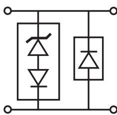
Optional Unidirectional configuration (TVS and separate rectifier diode in parallel)
