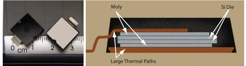
PLAD provides large exposed metal pads on the bottom of the package with excellent direct internal connection to the die (15KP and 30KP family packages shown).
